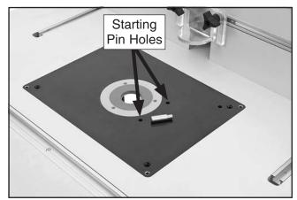
Figure 10. Proper location of the starting pin holes.
